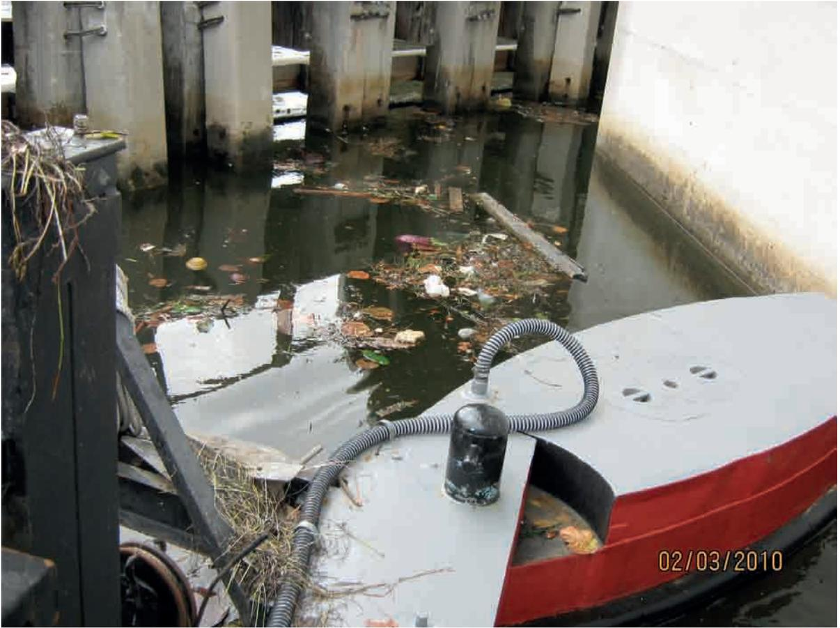
Scavenger2000 normal operation removing debris
